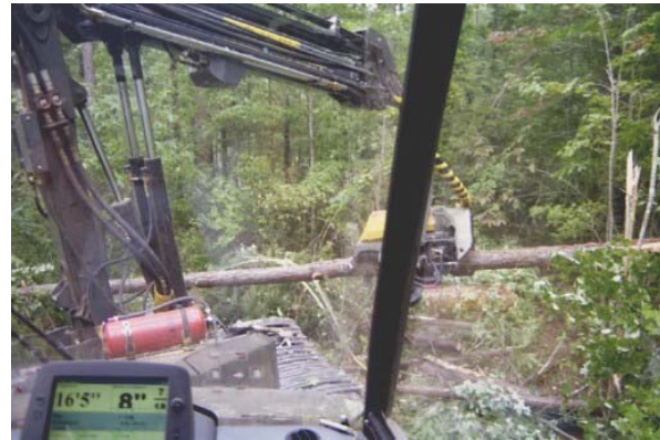
Photo 4. View from the harvester's cabin with the screen of optimization computer system is the lower left corner of the photo.
